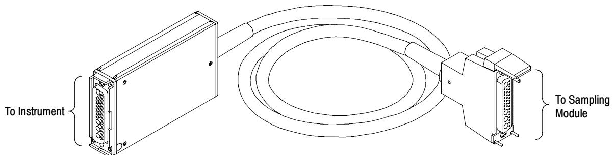
3. Use the connector marked “To Sampling Module” to connect to the sampling module. See the sampling-module user manual if you require information on connecting signals to the sampling module.
